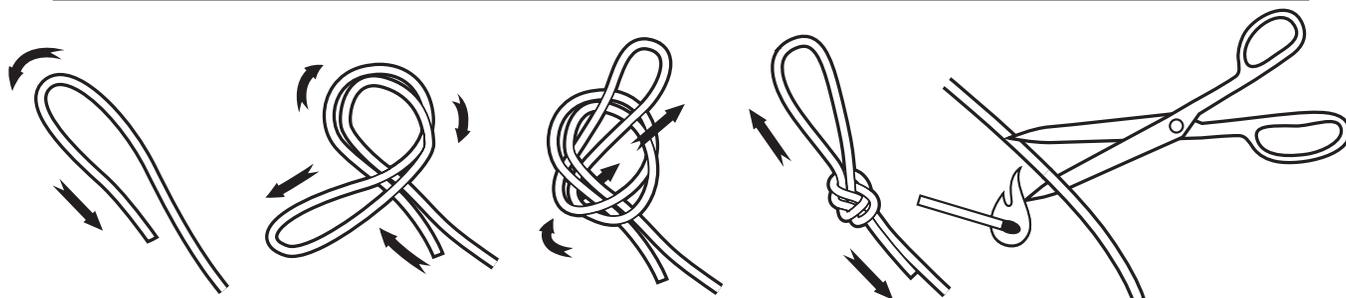
CUT UNDESIRED LENGTHS (OPTIONAL). FLAME TREAT ENDS OR CUTTING AREA WITH MATCH OR LIGHTER TO KEEP CORD FROM FRAYING. USE CAUTION WHEN WORKING WITH FIRE.
