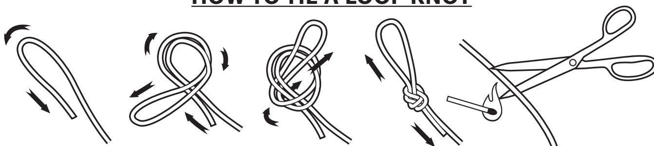
CUT UNDESIRABLE LENGTHS (OPTIONAL). FLAME TREAT ENDS OR CUTTING AREA WITH MATCH OR LIGHTER TO KEEP CORD FROM FRAYING. USE CAUTION WHEN WORKING WITH FIRE.
