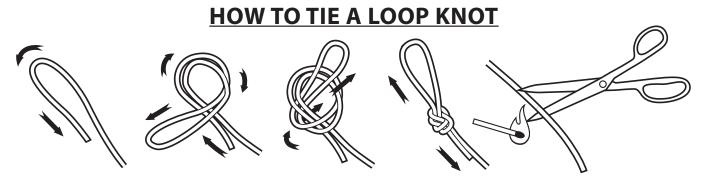
CUT UNDESIRED LENGTHS (OPTIONAL). FLAME TREAT ENDS OR CUTTING AREA WITH MATCH OR LIGHTER TO KEEP CORD FROM FRAYING. USE CAUTION WHEN WORKING WITH FIRE.
