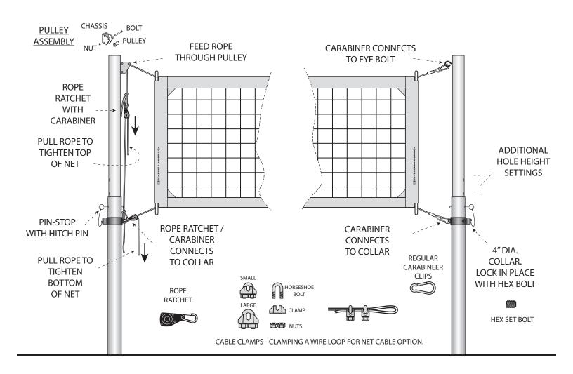
LOOSEN NET AND PULL HITCH PINS TO ADJUST POLE AND NET HEIGHT.
