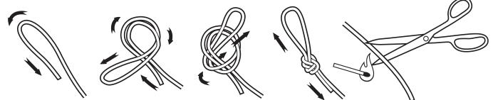
CUT UNDESIRED LENGTHS (OPTIONAL). FLAME TREAT ENDS OR CUTTING AREA WITH MATCH OR LIGHTER TO KEEP CORD FROM FRAYING. USE CAUTION WHEN WORKING WITH FIRE.
